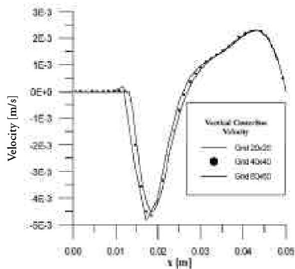
Figure 4. Vertical centerline velocity v/s grid size at  $t=50$  s.
