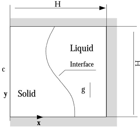
Figure 1. Scheme of liquid-solid phase-change problems in square section.
