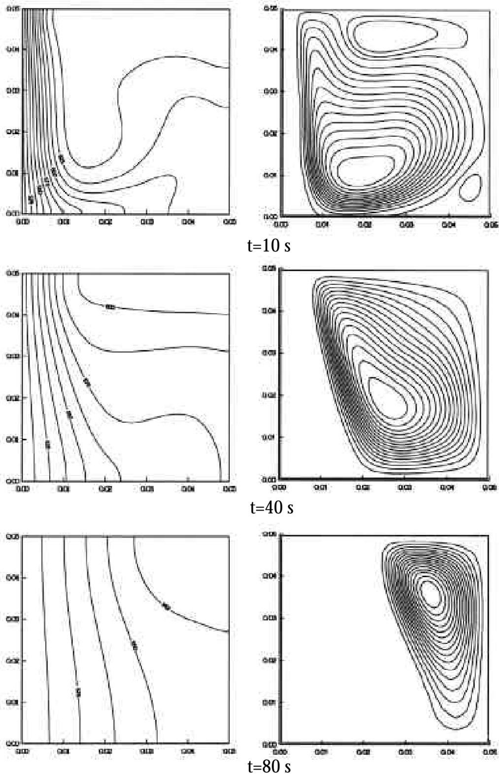
Figure 6. Isotherms and streamline for alloy aluminum solidification.
