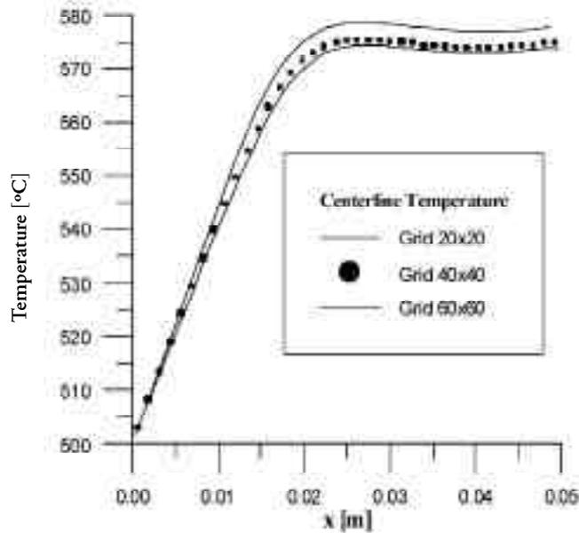
Figure 3. Centerline temperature v/s grid size at t=50 s.
